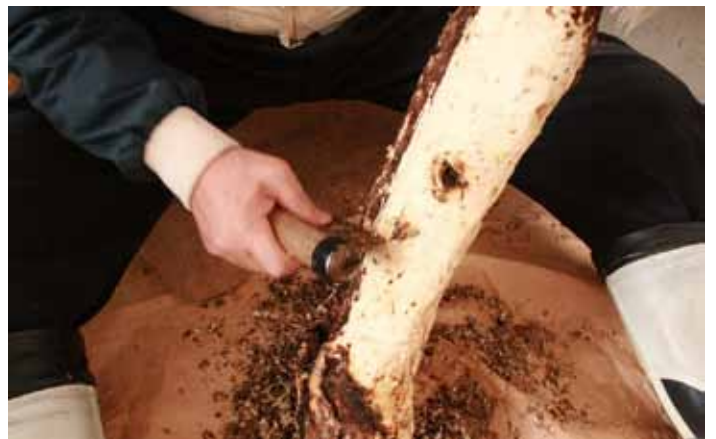
Scraping the root to produce the neri
