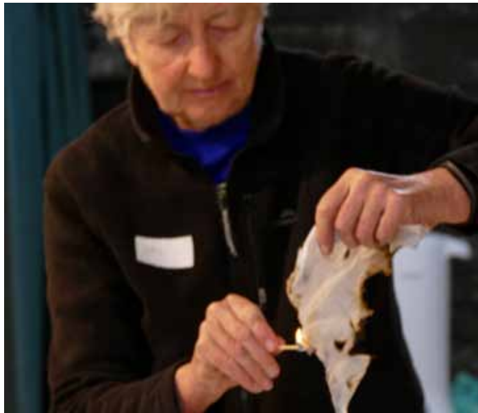
The burn test
