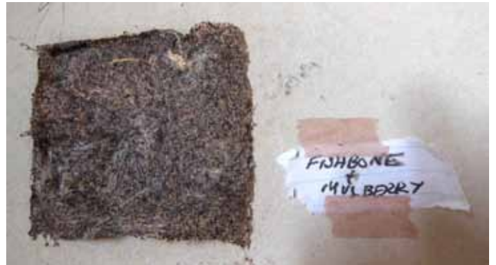
Restraint drying a sample of fishbone fern and handbeaten mulberry paper on cement sheeting
