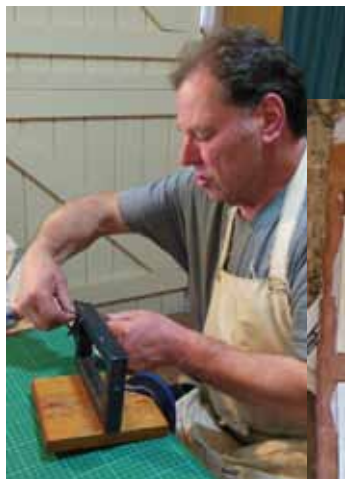
Jim using the paring device and the tools for making holes in the cover
