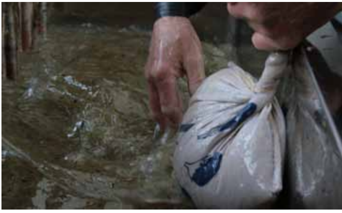
The viscous neri is squeezed into the vat of water and fibre
