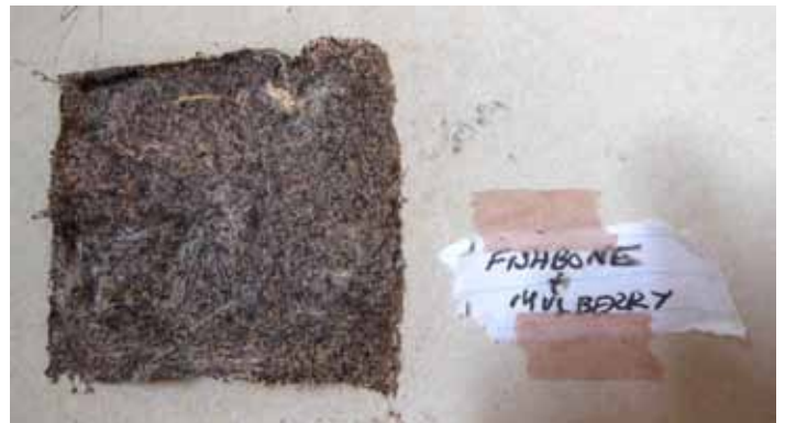
Restraint drying a sample of fishbone fern and handbeaten mulberry paper on cement sheeting
